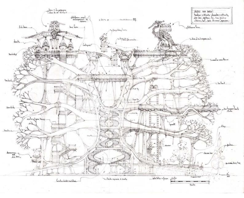
This steel and wooden tree will measure 50 m (165 ft.) in diameter. It will stretch 32 m (105 ft.) in the air and will be made up of 22 branches, resulting in a kilometrelong stroll in the air, half of which is in the incredible hanging gardens. Just like the Grand Éléphant, the Heron Tree will be an urban machine that is accessible to all that can be observed and visited however one likes.
