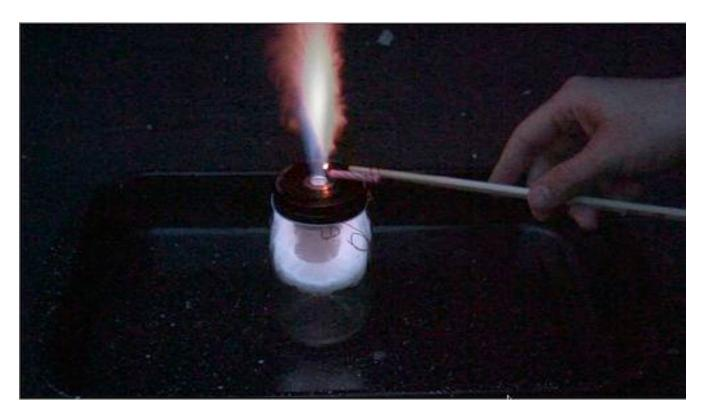
I had a few challenges along the way. I couldn't get ahold of a canning jar, and so I used a very similar jam jar. This worked pretty well but not as well as if I had used a canning jar. The copper tubing was a bit different too and I ended up just using one piece instead of two.
