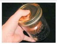
NOTE: When you remove your finger from the hole, you should notice a slight pressure release, and the jar should make a very faint "pfftt" sound. If you teel no slight pressure and hear no sound, shake the jar again. If there is still no pressure, there is a leak in the seal of the jar that you'll need to fix.
